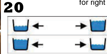
If desired: Add flush direction decal to the front of tank behind the handle. note: the "small" rinse flush is always toward the outside.
