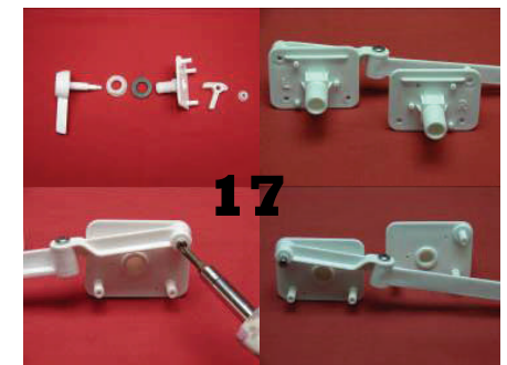
Transfer lever arm assembly from the left to the right plate by unscrewing lever arm assembly on the left plate and screwing it on to the right plate.
